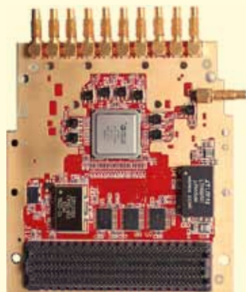
Рис. 1. Модули Vita 57.1 (FMC) Quad 12-Bit (4 GSps) ADC Quad16-Bit (12 GSps) DAC Module
